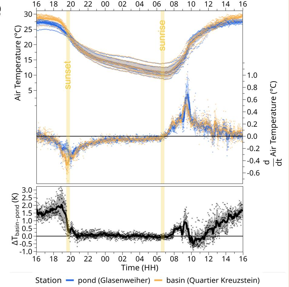
The two sites basin and pond are separated by a 8 to 10 m high dam (distance ≈ 80 m) and are characterized by different microclimates. During the day, the cooling effect of the pond was limited by the dam.
