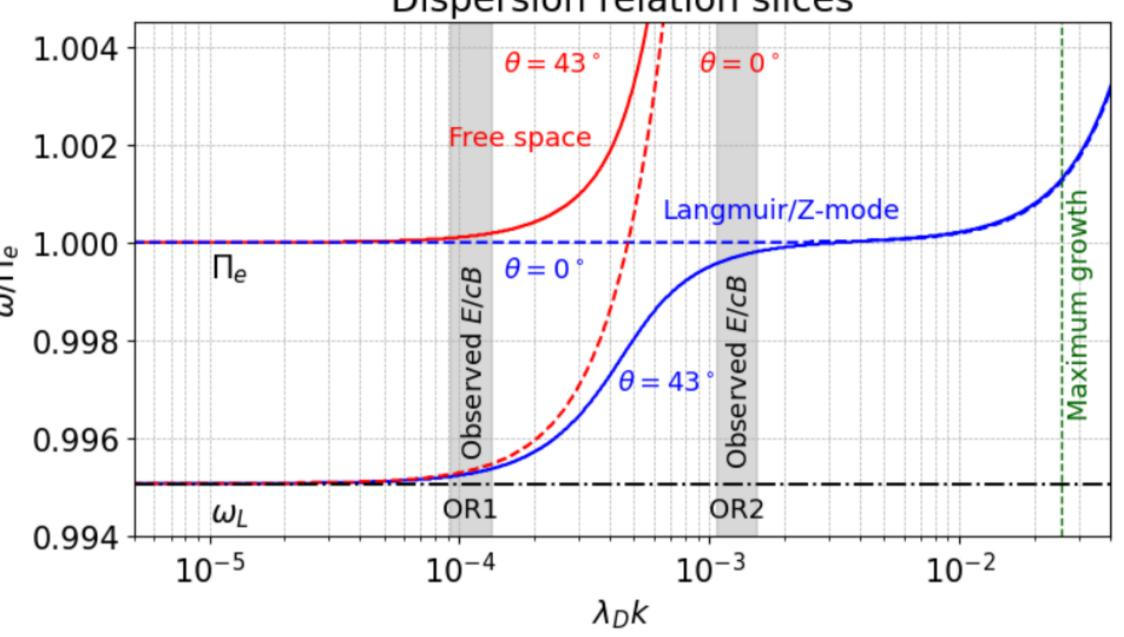
Figure 7: (Top): Wave growth rate for a modified distribution. (Bottom): Dispersion relation of the Langmuir/Z-mode and the free space L-O mode with wavevectors parallel (dashed lines) and at  $\theta$ =43° (full lines). Regions highlighted in gray correspond to the observed ratio of the E/cB fields.
