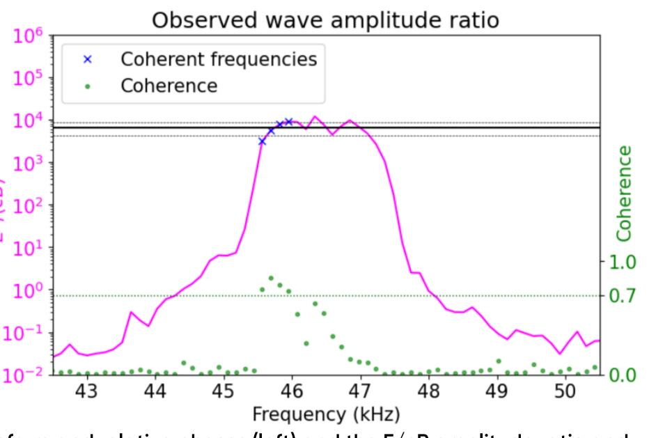
Figure 8: Waveform measurements from 13:52 UT showing the waveform and relative phases (left) and the E/cB amplitude ratio and signal coherence of the same waveform snapshot (right).
