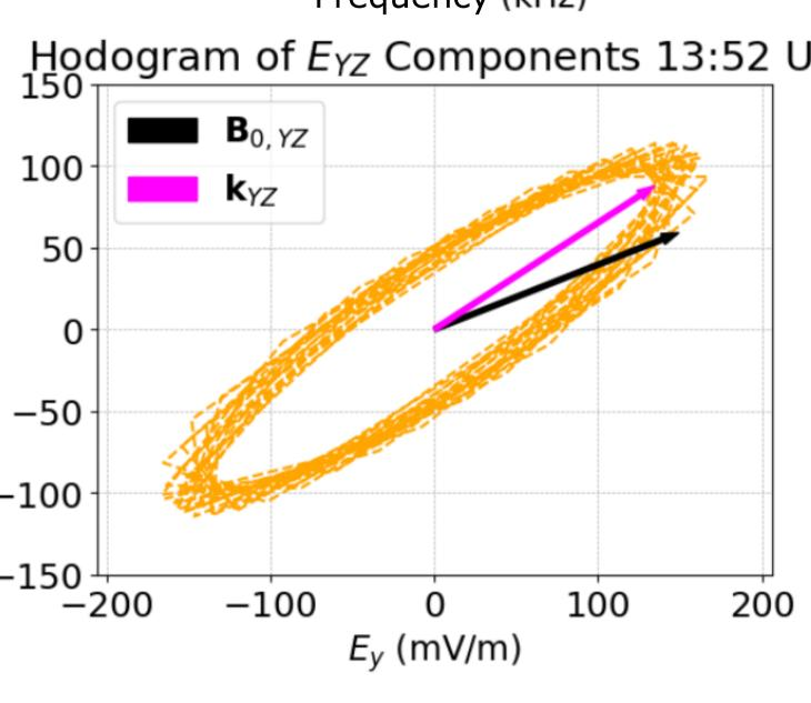
Figure 5: Top: spectrum of the waveform recorded during the middle timestamp of 13:52 UT. Bottom: hodogram of the peak amplitudes within the waveform observed at 13:52 UT with the direction of the background **B** field (black) and predicted wave vector direction (purple).
