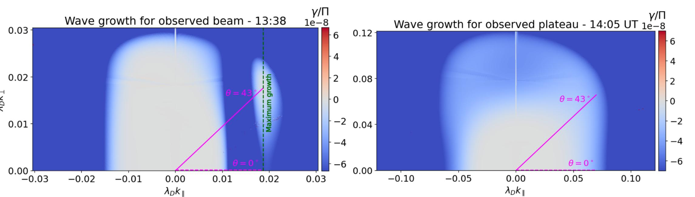
Figure 6: Wave growth obtained from WHAMP for the observed distributions at 13:38 and 14:05 UT. The purple lines highlight wave vector angles - the 43° angle corresponds to the maximum growth rate at 13:38 UT. The green dashed line corresponds to the Landau resonant  $k_{\parallel}$ .
