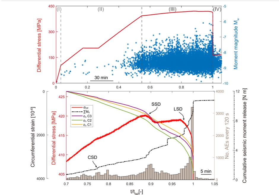
Fig. 3. (Top) Differential stress (red line, left axis) and the moment magnitude of the AEs (blue dots, right axis) as a function of time. (Bottom) Differential stress (red line, left axis), mean strain for each DSS line (yellow line: bottom level; green line: middle level; purple line: top level, left axis), number of AEs at two-minute intervals (histogram bars, right axis) and cumulative seismic moment (dashed line, right axis) during Phase III.
