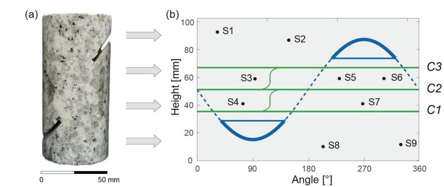
Fig. 2. (a) Rotondo granite sample with a pair of 15 mm deep notches at a 35° from the loading axis. (b) Projection of the PZT (black dots) and DSS (acrylate fiber in green) sensor positions on the sample surface.
