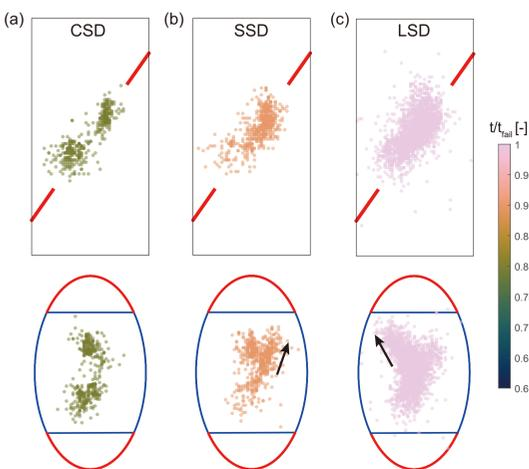
Fig. 4. Sequence of AE locations obtained within a 60 s window starting ~15 s following the nucleation of a slip event. The slip events are shown in parentheses. The top row shows the locations in the depth plane, and the bottom row shows the same locations projected on the fault plane. The black arrows indicate the direction in which the AE clusters are spreading.
