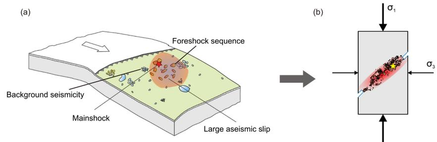
Fig. 1. (a) Schematic of the aseismic slip and earthquake sequences for the 2009 M5.8 earthquake in northern Peru [3]. (b) Schematic of aseismic deformation and acoustic emission (AE) events during the triaxial rock experiment.
