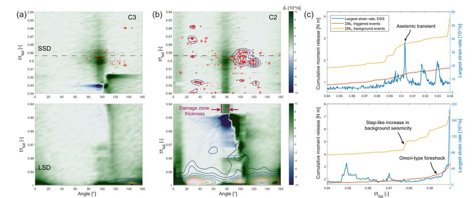
Fig. 6. (a, b) Strain rate based on DSS data for circumferential cable C3 (a) and C2 (b) with triggered events superimposed. The contour plot marks the density of events. (c) Cumulative moment release of background seismicity (orange line, left axis) and triggered events (red line, left axis), largest strain rate (blue line, right axis).
