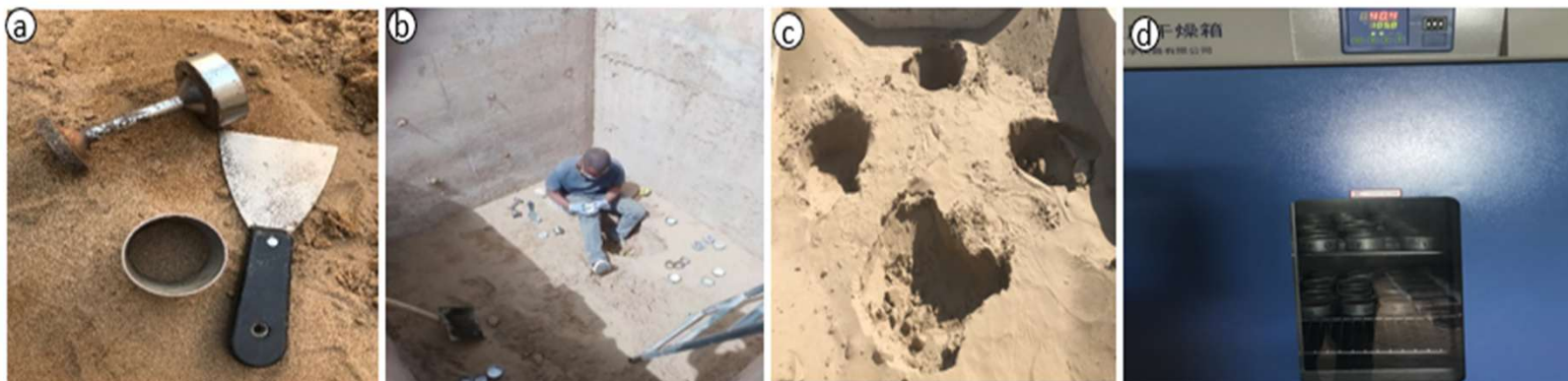
a) Core rings and knife b and c) Soil sampling design in a tank and d) Oven dry with soil core.
