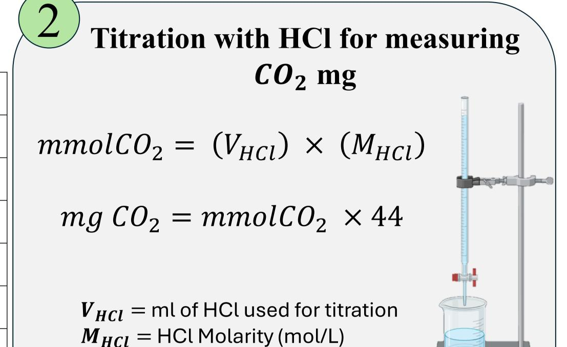
Measurement of the % of biodegradability of PLA through CO<sub>2</sub> emissions
