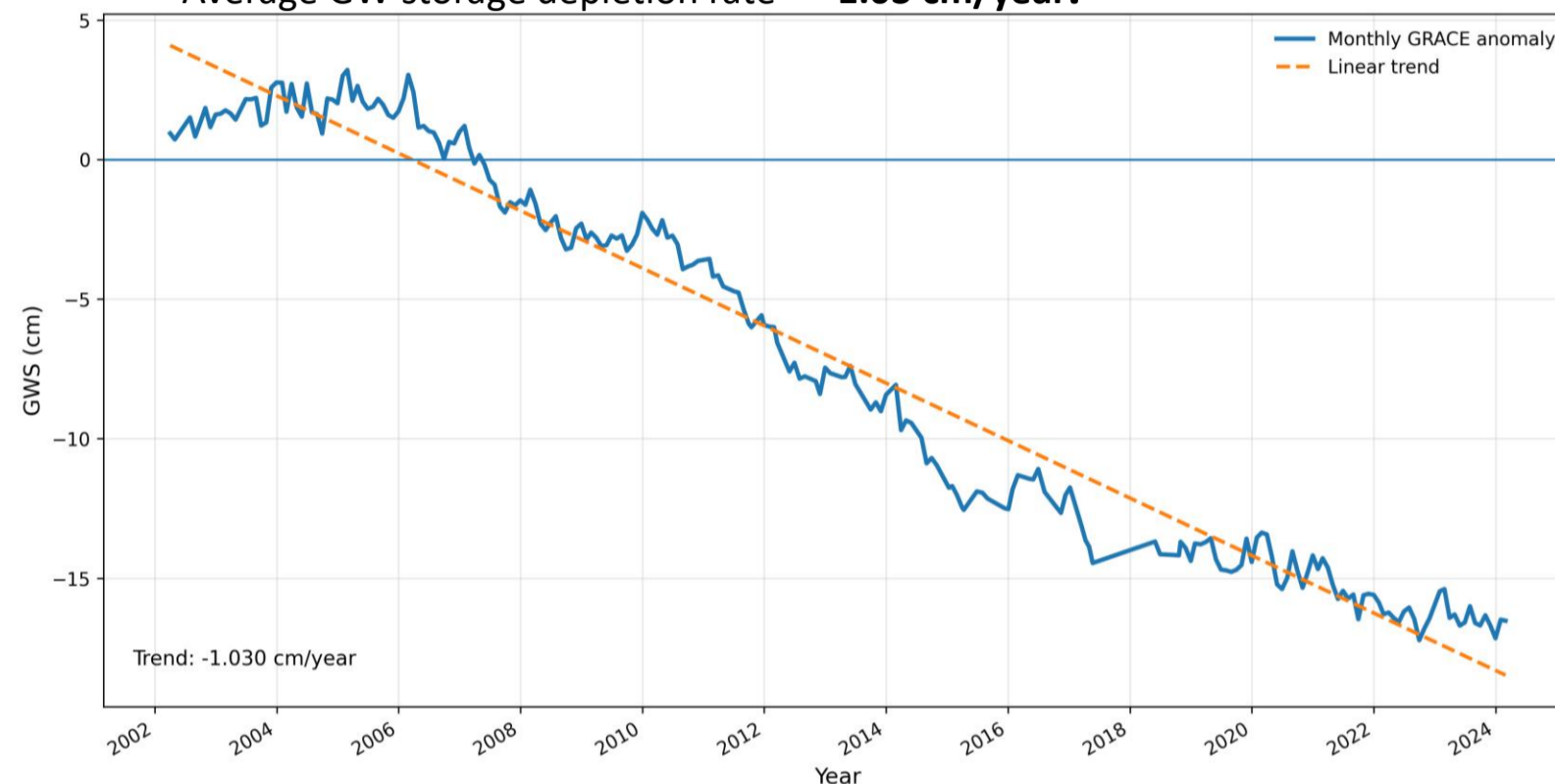
Fig. 2: GRACE-derived Groundwater storage change in heavy extracted region of Saudi Arabia for 2002-2024.
