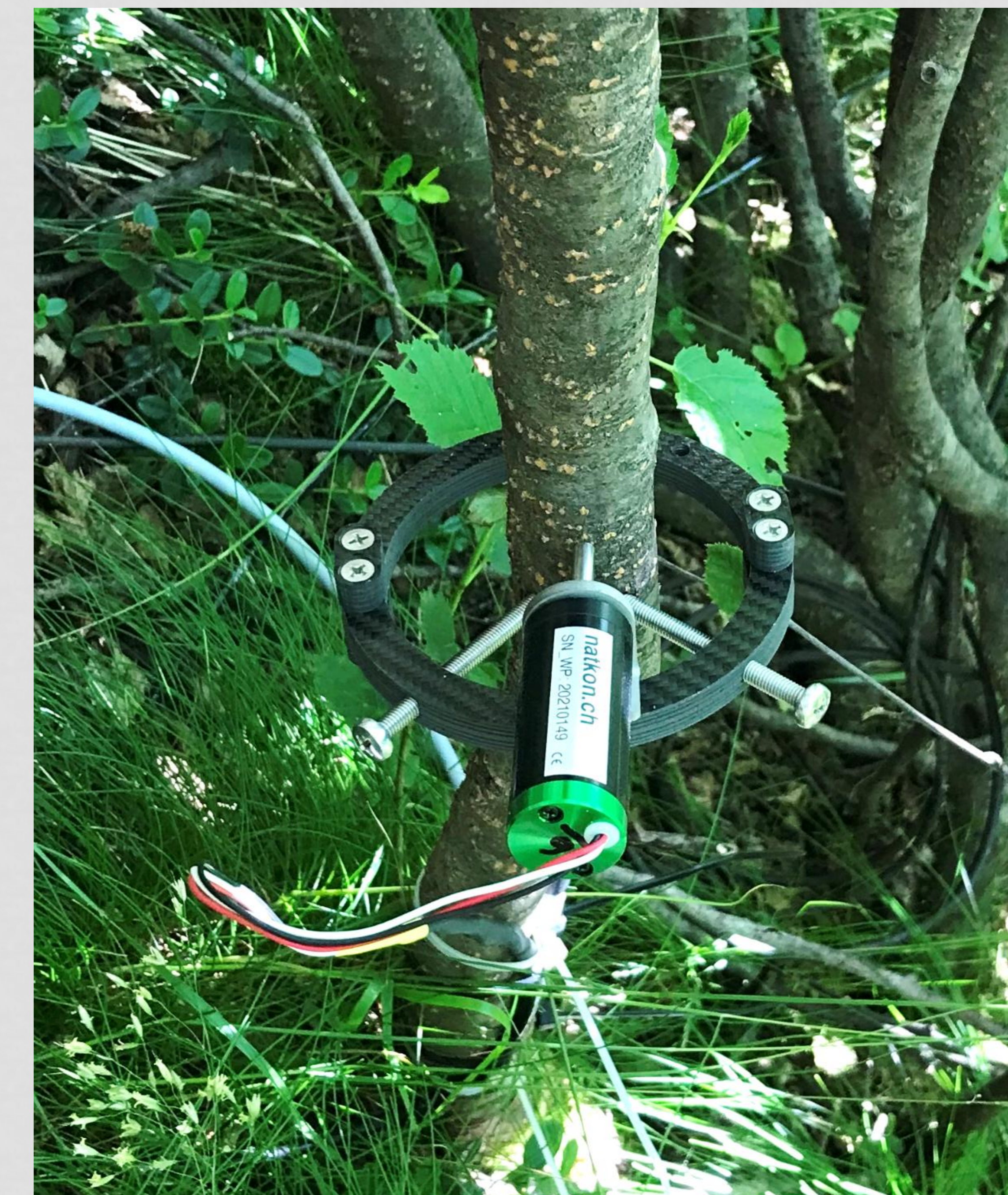
Point dendrometer mounted on the stem of Alnus alnobetula (ZN12-O-WP, Natkon.ch, Switzerland)
