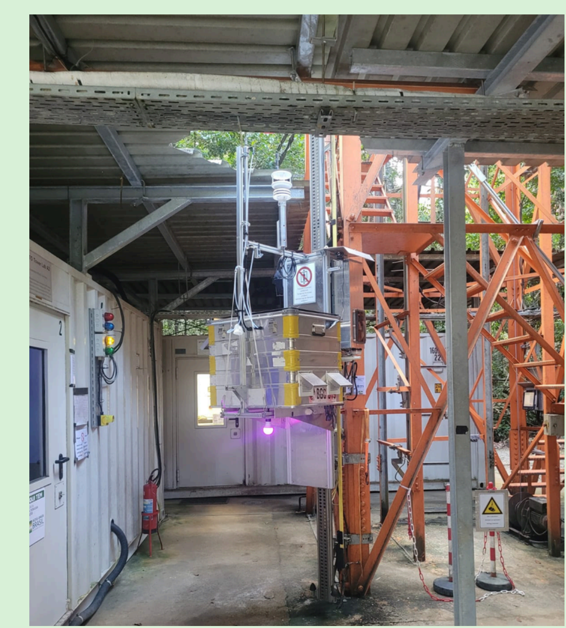
Figure 1: RoLi lift and instrument box on the ATTO tower.
