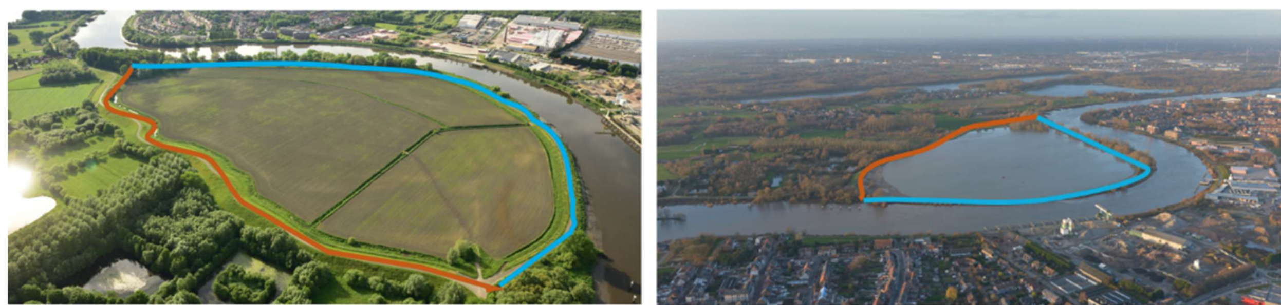
Controlled flood area under normal conditions (left) and storm tide (right). Red indicates the ring dike, and blue indicates the overflow dike.
