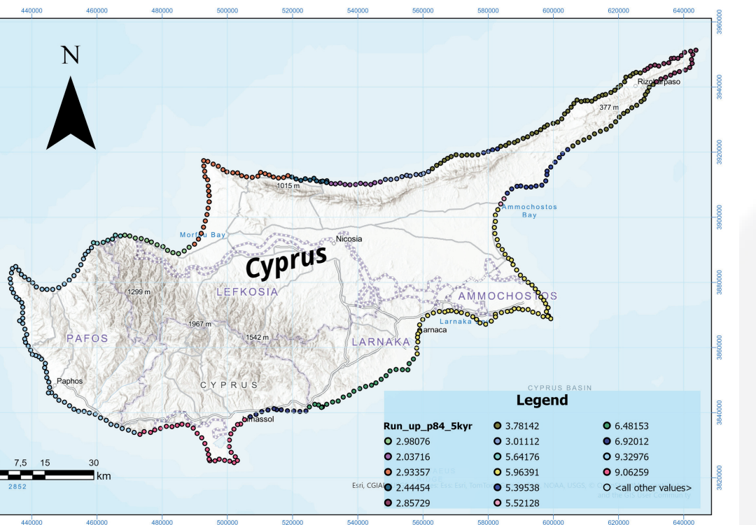
Figure 5: Example of coastline segmentation of Cyprus and conversion of MIH values at POIs to run-up points along the coast, using a dedicated Python tool.
