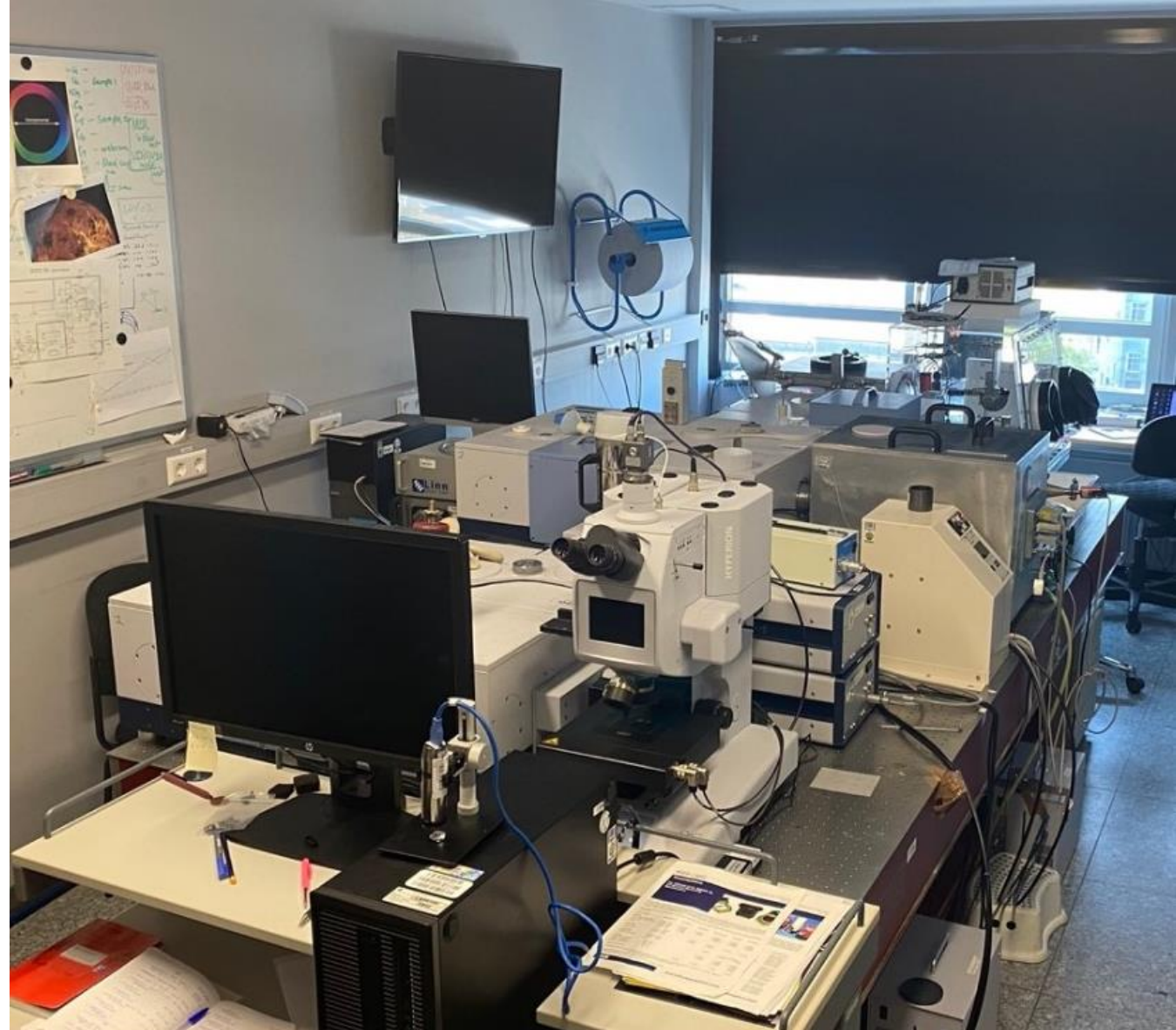
The Planetary Spectroscopy Laboratory and its external units: Hyperion microscope, the emissivity chamber and the cryochamber (modified after Helbert et al., 2024)
