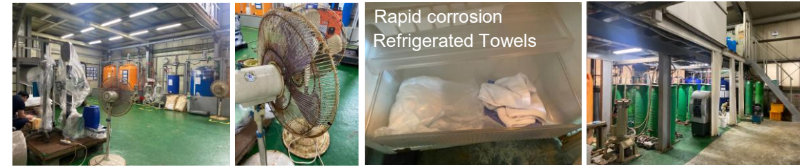
▲ Chemical: Internal heat + limited ventilation → Heat stagnation and amplification
