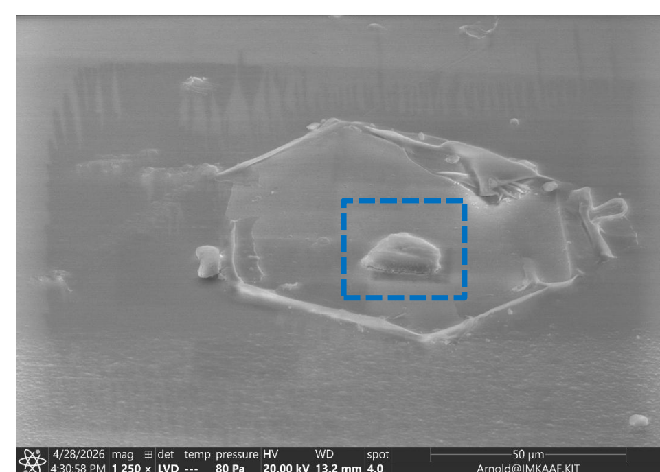
Replica of a plate ice crystal. The particle found within the replica shows K and N peaks similar to the EDX-spectrum shown above.
