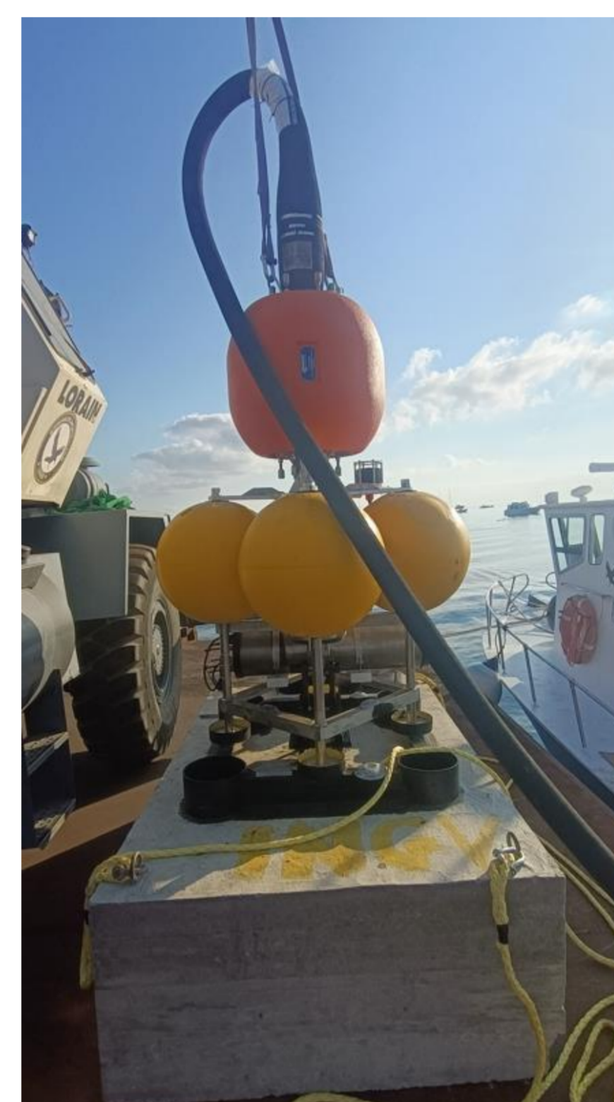
Fig. 3 The seafloor module anchored to a reinforced-concrete deadweight.
