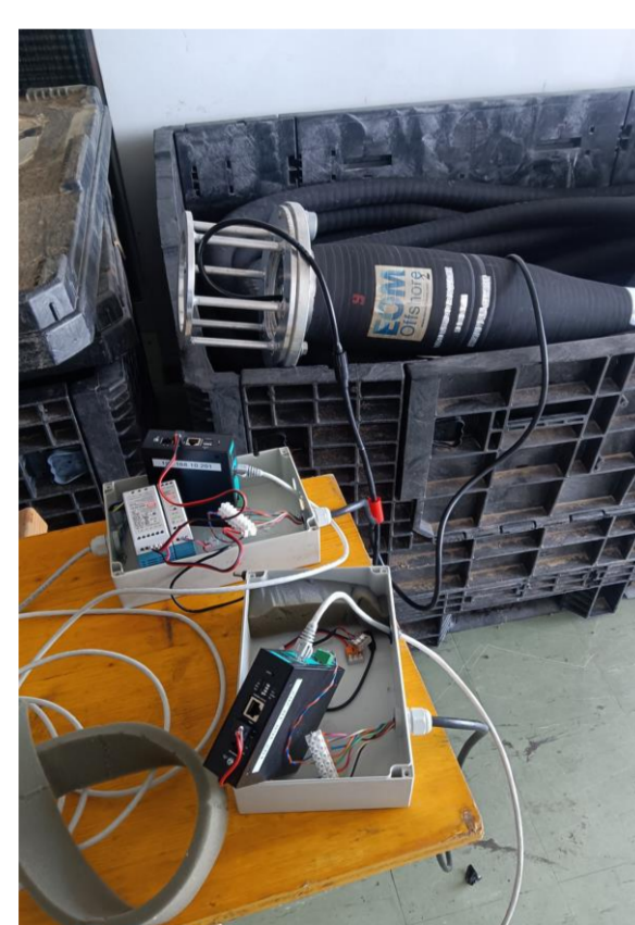
Fig. 7 Electrical transmission tests before and after force-extension test.
