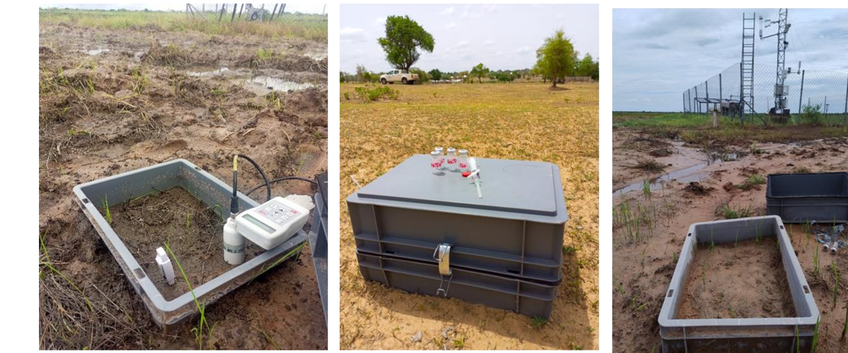
Fig. 2: Chamber-based greenhouse gas sampling plots; closed (middle) and opened (right).
