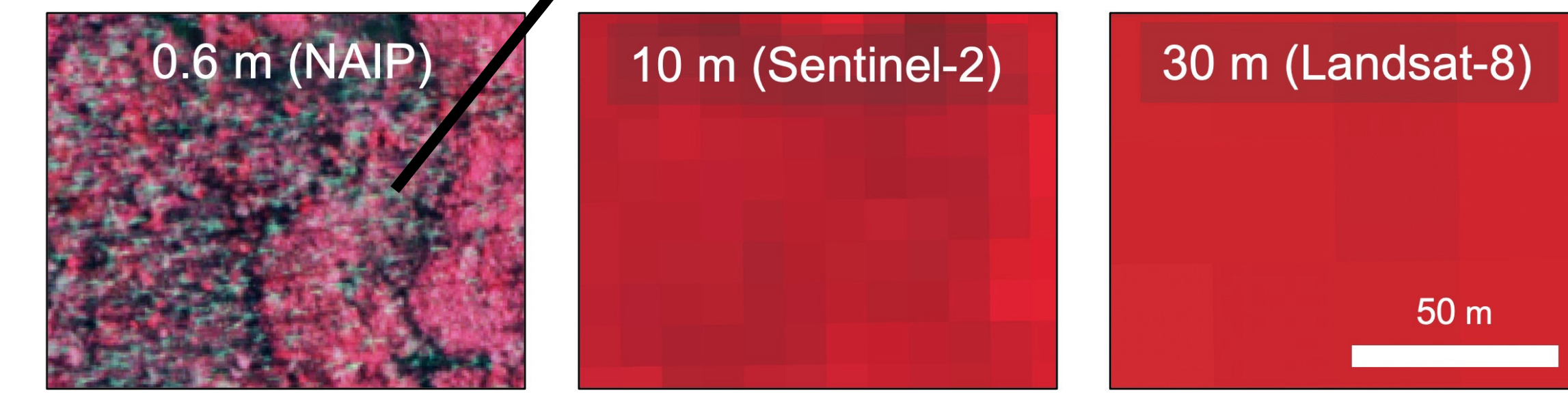
Fig. 2 | Coarser-resolution satellites severely underestimate coastal tree die-offs. False-color images where dead trees and healthy vegetation are displayed in white/grey and red, respectively (Yeung et al. 2025, Nat. Sustain. )
