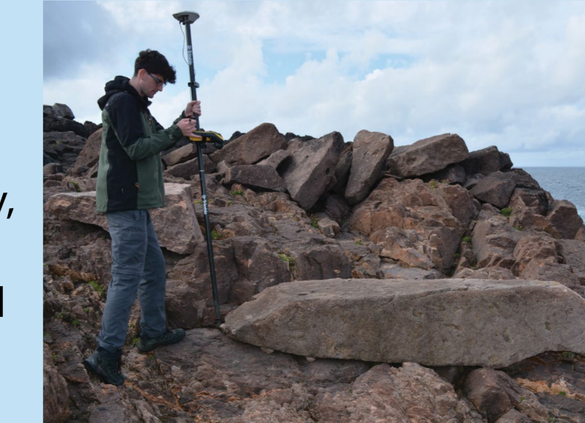
Fig. 9., Field photograph of traditional boulder measurement including taking DGPS measurements.
