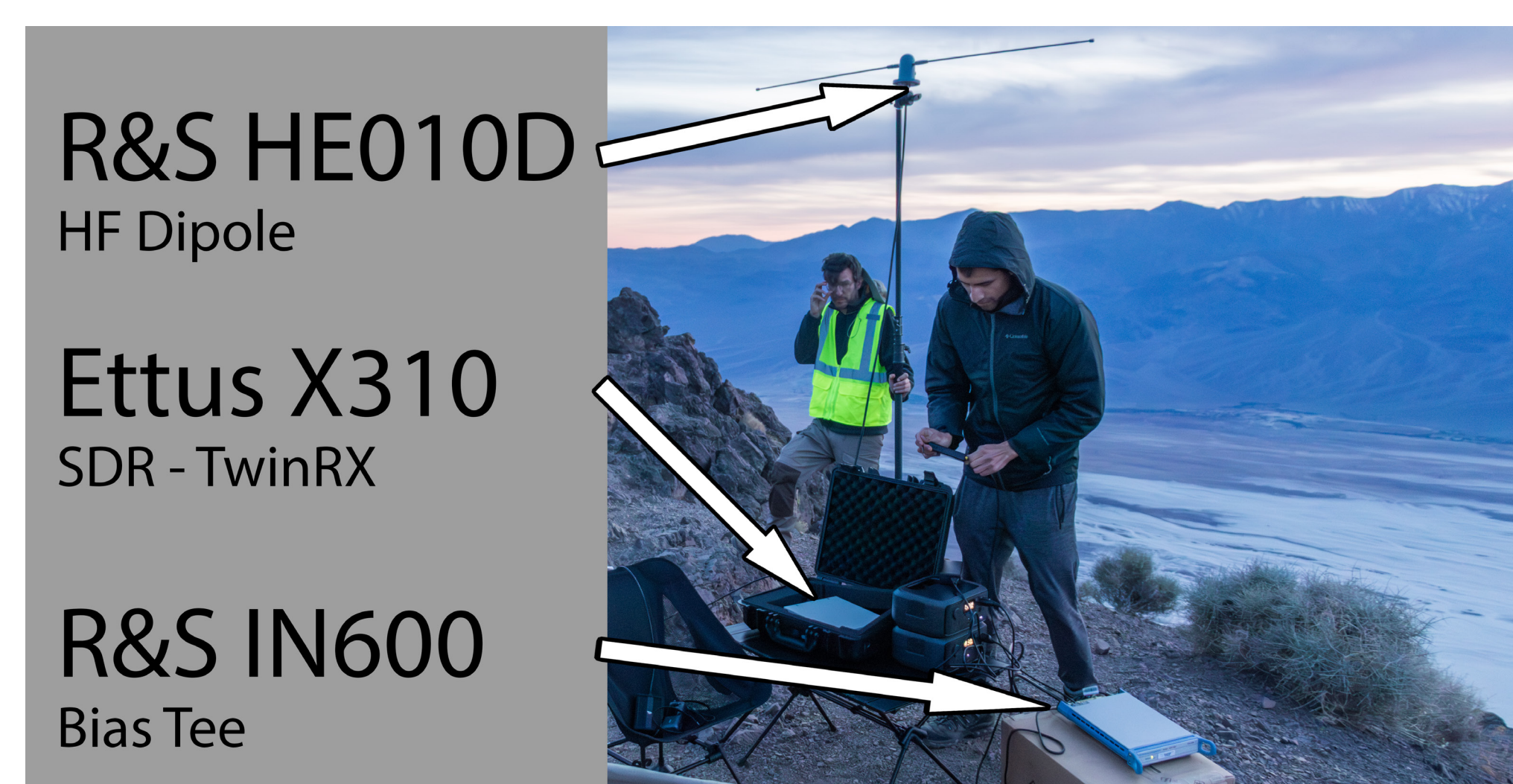
Fig. 2: Experimental setup and hardware.
