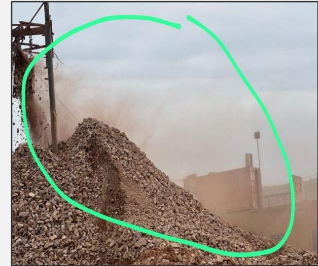
Figure 10: Dust generation during ore processing, illustrating exposure to respirable particles in artisanal mining.
