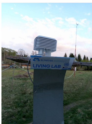
Figure 3.2 – Photographs of the Arduino-based air quality monitoring station installed at the Slavsko meteorological station
