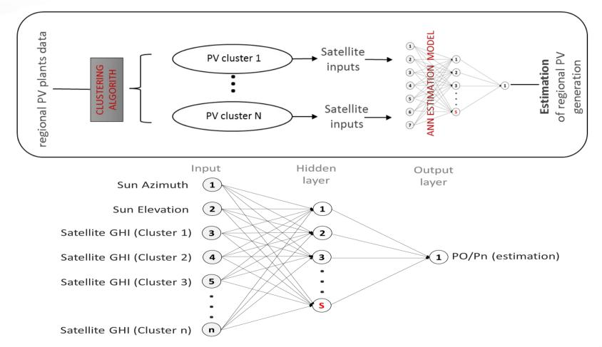
The power estimation model achieves, using satellite derived irradiance, an RSME of 3% of the installed capacity and a MAE of 2%.
