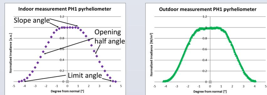
The PH1 pyrheliometer angular response or effective penumbra function was measured in the lab and outside. In the lab a lamp and an angle indicator was used. Outside the PH1 was pointed to a point where the sun would pass at a later moment and then measured over time. The measured slope angle, opening half angle and limit angle [6] are in good agreement with the expected values of 1°, 2.5° and 4°.
