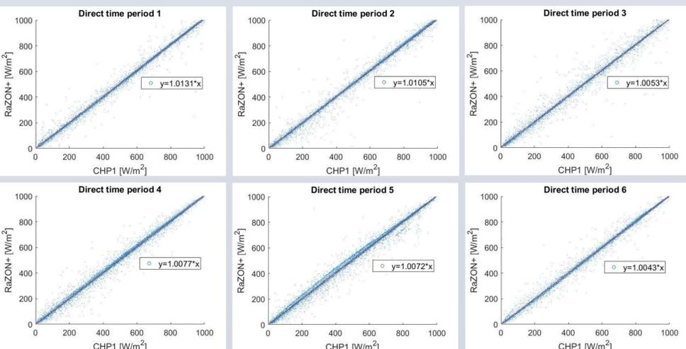
The data has been cut into 6 blocks of approx. 3 months. For each block the DNI of the PH1 is plotted vs the reference irradiance measured by the CHP1. The change in slope is due to built up of soiling. The slope changes from 1.013 to 1.004.
