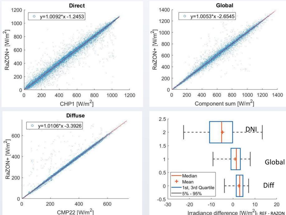
The comparison of the RaZON+, with the reference system is shown above.
