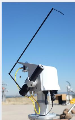
The RaZON+ is a cost effective solar monitoring system with internal datalogger and GPS.
