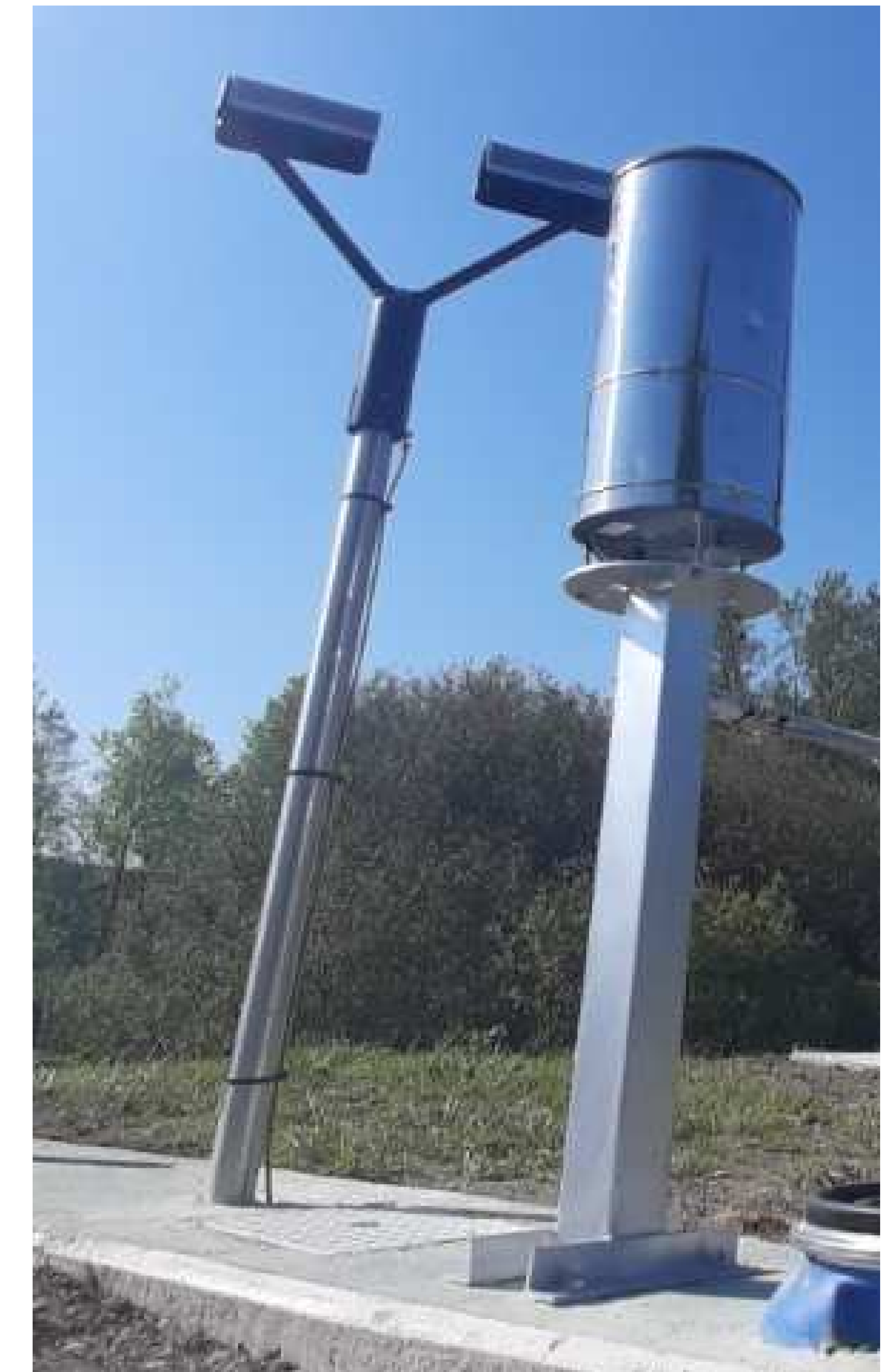
An example of disdrometer ( dis ) and tipping bucket rain-gauge ( tbg )
