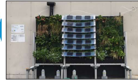
Non-ground-based PV-driven and irrigated VertiKKA greening modules, New parameterization developed for ENVI-met modelling
