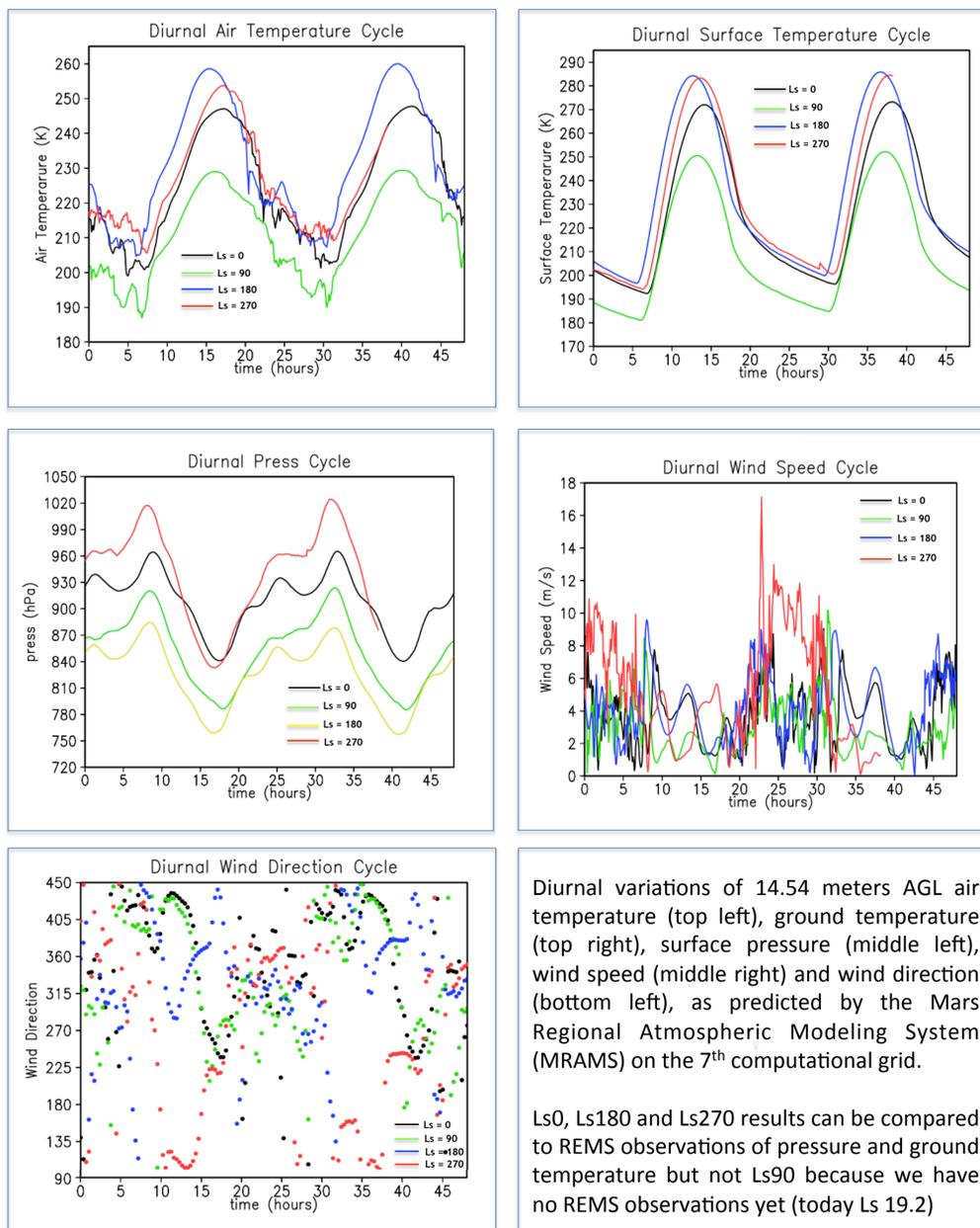
Diurnal variations of 14.54 meters AGL air temperature (top left), ground temperature (top right), surface pressure (middle left), wind speed (middle right) and wind direction (bottom left), as predicted by the Mars Regional Atmospheric Modeling System (MRAMS) on the 7<sup>th</sup> computational grid.
