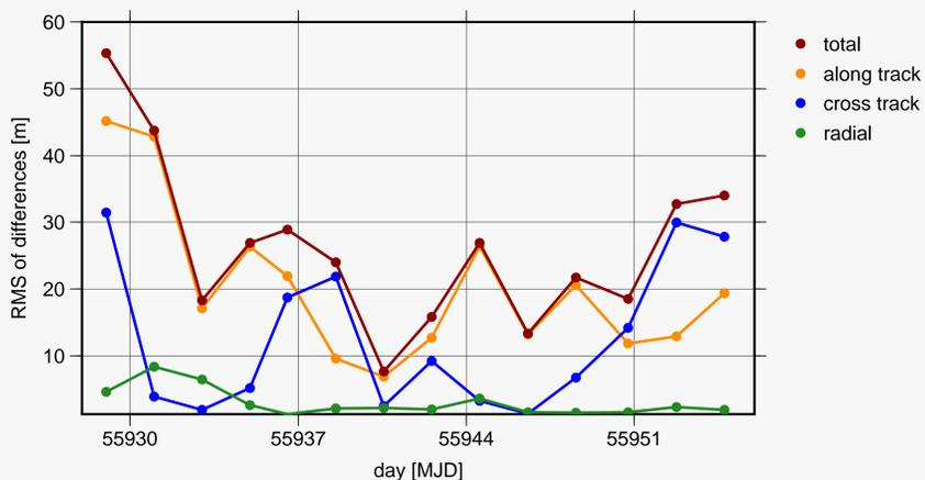
Fig. 3: Differences of 14 orbit arcs from laser and Doppler data to NASA orbits (January 2012, arc length 2.5 days).
