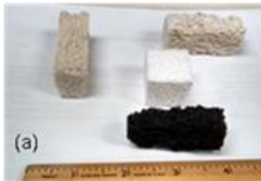
Sample materials: a) alumina foam, b) kaolinite clay, c) Murchison CM2 in alumina
