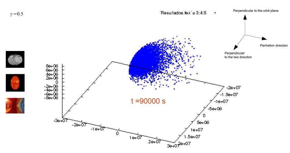
Position of 10000 particles subject to the asteroid and sun gravitational field as well as the sun radiation pressure. Considering  $\theta$ =0,  $\phi$ =0, h=10 m, step = 0.8 s ,  $\rho$ =1000 Kg/m3 y t = 90000 s. View (139, 336), xrange (-30000000, 30000000), yrange (-20000000, 20000000), zrange (-9000000, 9000000).
