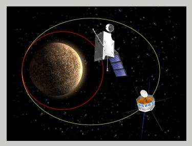
For **nominal** operations, the **Z-axis** is aligned with the **NADIR** direction.
