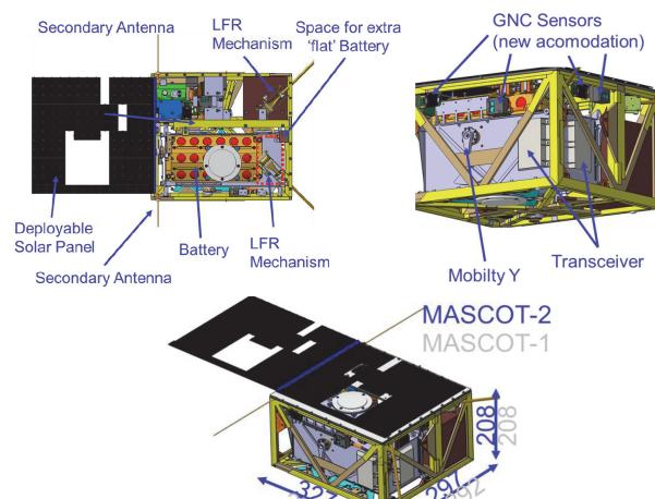
Figure 2 – MASCOT2 design. Note that all faces are covered with solar cells
