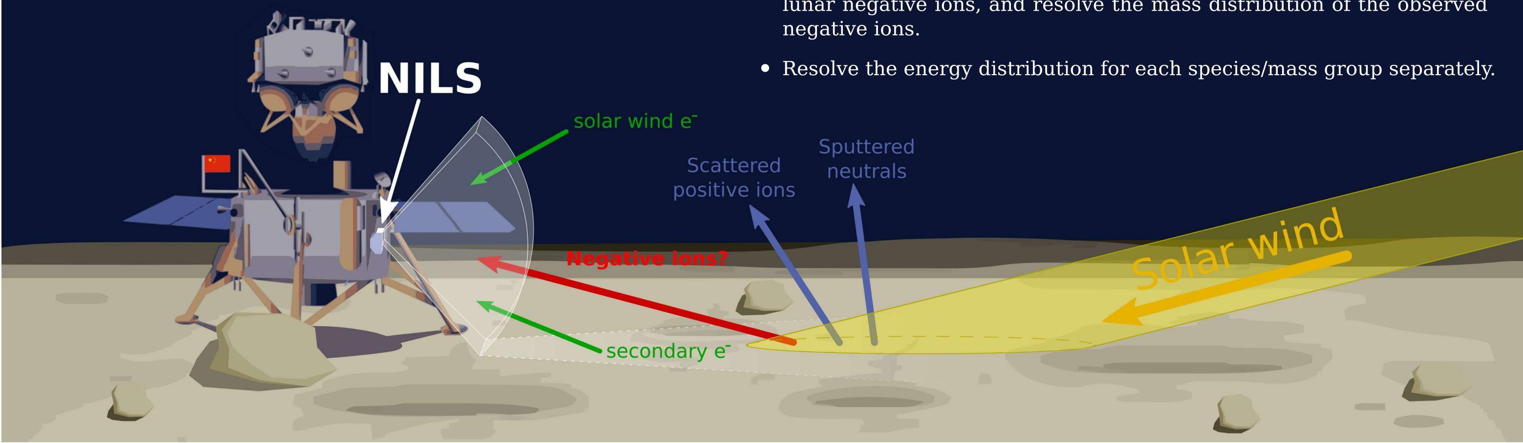
Previous in-situ measurements beyond the Earth relied on energy spectrum information [1,2,3]. How to unambiguously separate negative ions from electrons?
