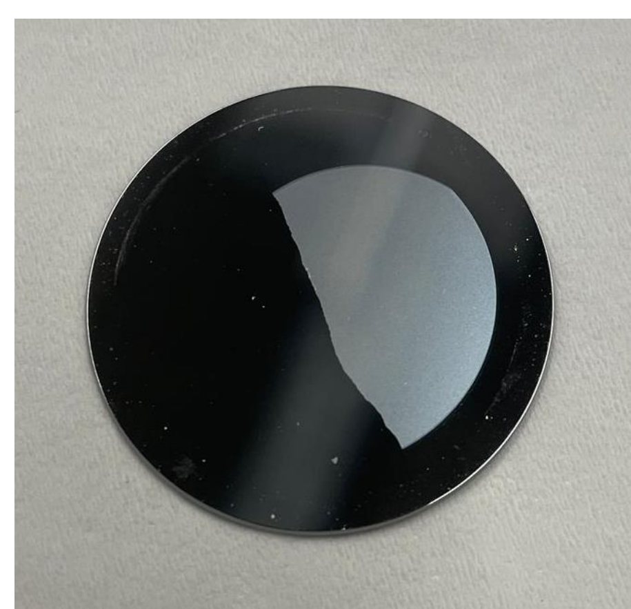
Ru substrate covered with MgFeSiO 4 (light gray area)
