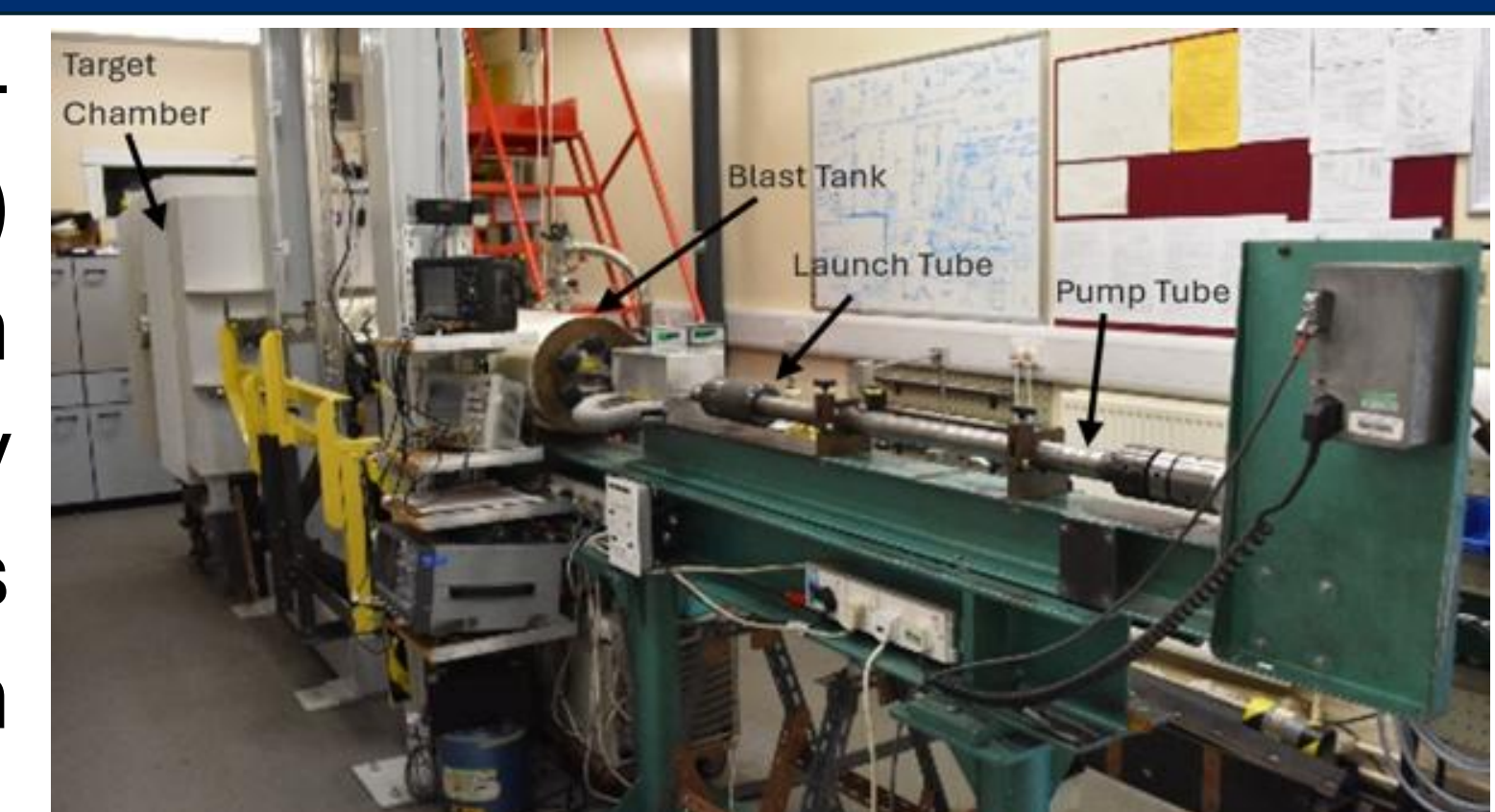
Figure 3: The University of Kent's Two-Stage Light Gas Gun.
