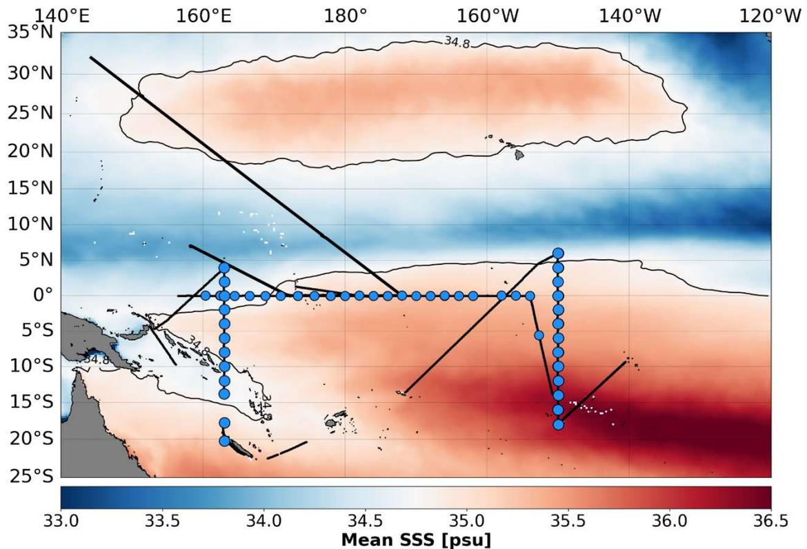
Figure S3. Sea Surface Salinity (SSS) averaged over the 5 surveys (sept/oct 2021 to 2024), from Copernicus Marine Product (Global Ocean Physics Analysis and Forecast; (European Union-Copernicus Marine Service, 2016). Use of monthly average.
