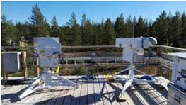
Brewer #037 has been operated in Sodankylä since May 1988. The instrument has been well maintained and frequently calibrated since to produce a high quality ozone time series now spanning over 27 years. In September 2012 a new double-monochromator Brewer was installed and after a difficult start has now been fully operational since November 2015.
