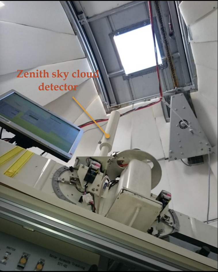
Photo 1. Umkehr measurements are made on a 7-degree cone of light emanating from the zenith sky.
