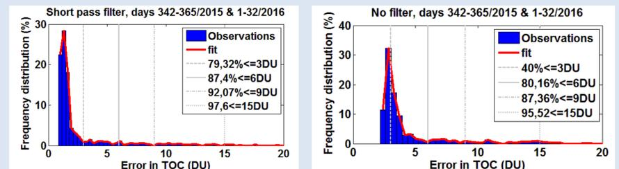
Figure 6: Frequency distribution of errors in TOC retrievals with (left) and without (right) the short-pass filter. The red line is a smoothing function fit and the vertical lines mark the percentage of data with error smaller than 3, 6, 9 and 15 DU.
