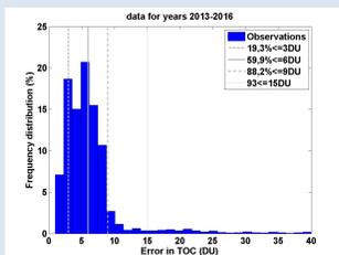
Figure 4: Frequency distribution of errors in TOC retrieval. The vertical lines mark the percentage of data with errors below 3, 6, 9 and 15 DU.
