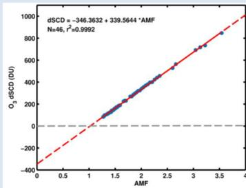
Figure 1: Example of a Langley extrapolation applied to the  $dSCD$ s derived from Phaethon direct radiance spectra recorded during 31/5/2015 at El Arenosillo, Spain. The constant term of the linear regression gives the  $-SCD_{REF}$  while the slope corresponds to the mean TOC of this day.
