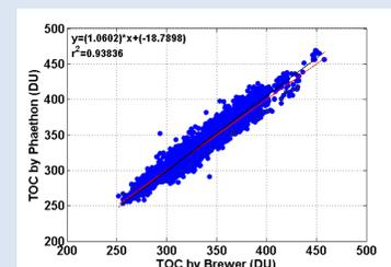
Figure 3: Scatter plot between TOC data derived by Phaethon and Brewer 005 with linear regression (black) and  $y=x$  line (red).
