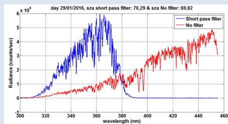
Figure 5: Example of direct-sun spectral radiance measurements recorded by Phaethon with (blue) and without (red) the short-pass filter, one after the other.
