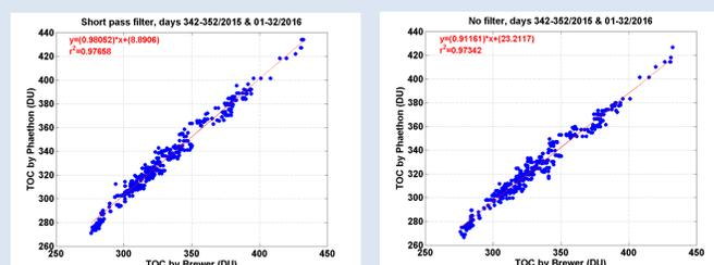
Figure 7: Scatter plot of Phaethon and Brewer derived TOC based on spectra recorded through the short-pass filter (left) and without the filter (right).
