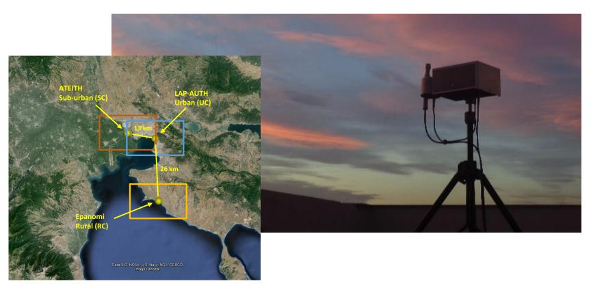
Three mini MaxDOAS systems Cooled miniature CCD spectrograph (AvaSpec-ULS2048LTEC) Operating since late 2013 in different locations Range: 300 nm to 452 nm Resolution: 0.34-0.42 nm Direct solar irradiance and sky radiance measurements (zenith and off-axis)
