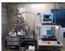
Fig.3) Millimeter-wave spectral radiometer at Syowa station.
