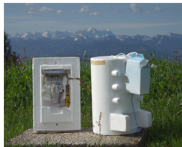
Brewer-Mast ozone sonde, 1997 (left, in Styrofoam box) with Vaisala RS80 pTU-sonde (blue box on the right)
