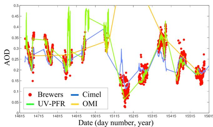
Above we show the AOD at 320 nm measured by the Brewer instruments during the campaign. For comparison, we have also included data from the AERONET AOD level 1.5 product of the Huelva station (shifted up by 0.07 because the lowest wavelength measured by this particular Cimel sunphotometer is 440 nm), the OMI OMAERUV level 2 overpass data at 352 nm from the Aura Validation Data Center [7], and the AOD measured at 320.1 nm by a UV-PFR instrument operated by the PMOD/WRC.
