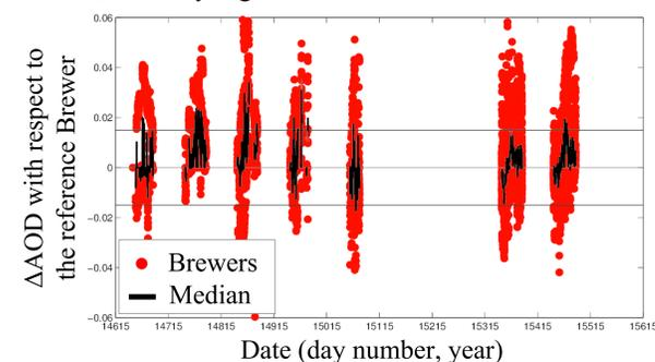
With the data from the campaign, we have also been able to calibrate the AOD. The figure above shows the AOD differences at 320 nm between participating instruments and the RBCCE reference Brewer. 93% of the medians of the differences are smaller than 0.015.
