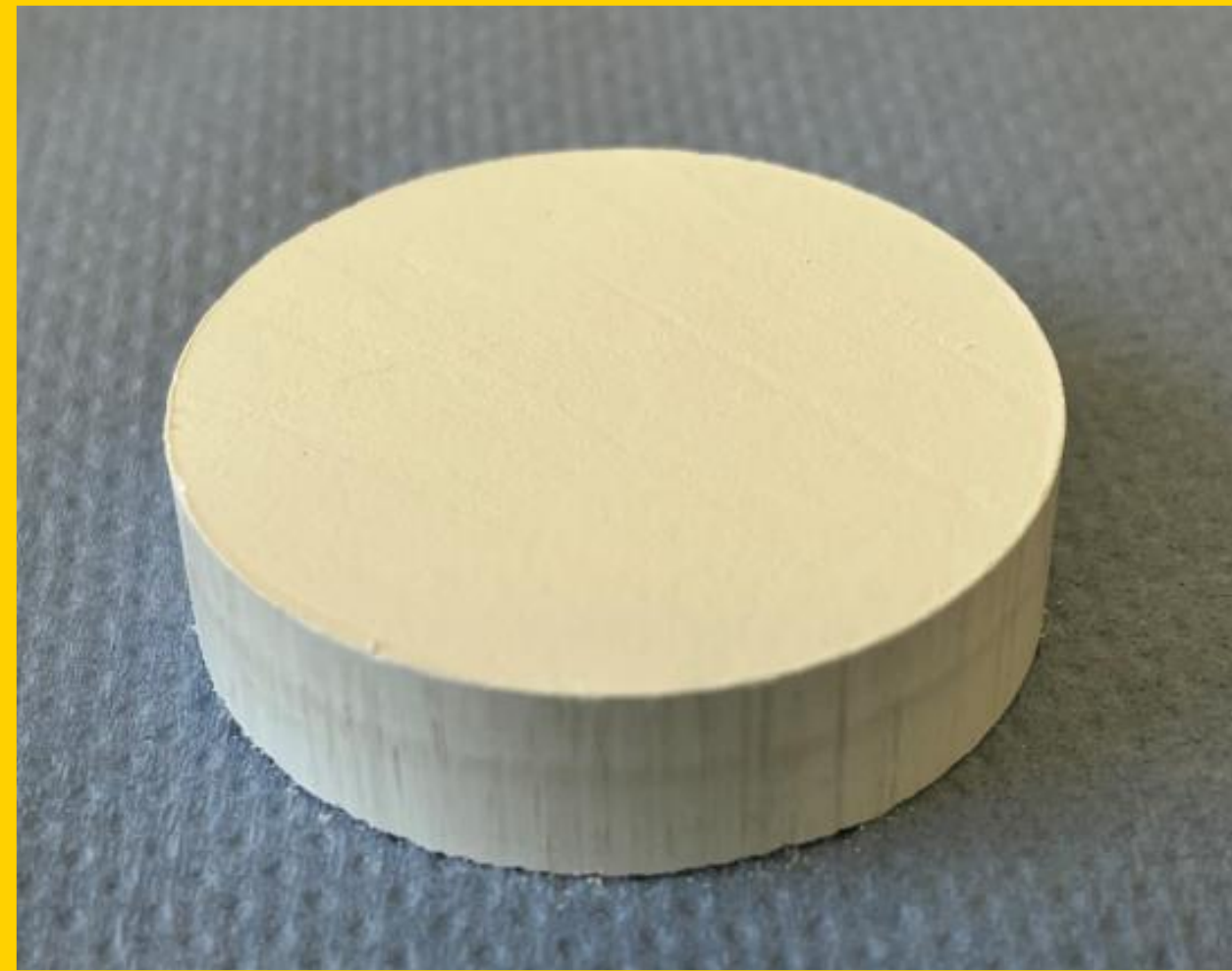
Fig. 1a: Plug after molding at 10 MPa.
