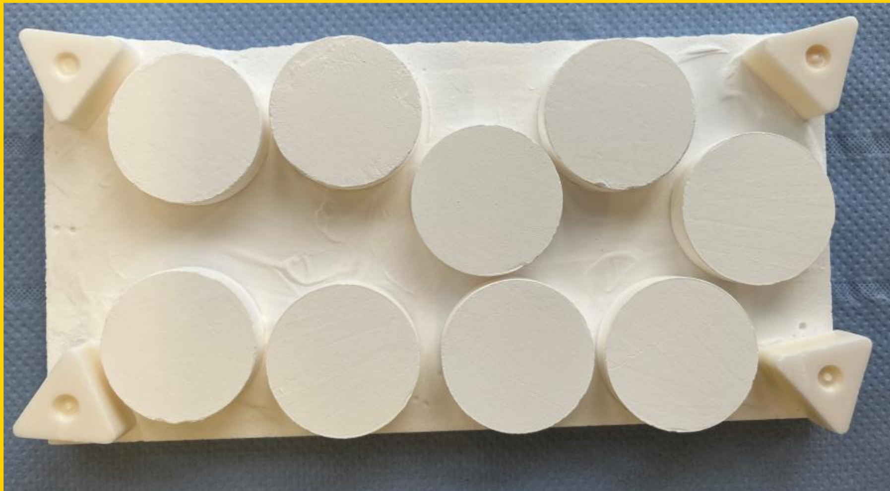
Fig. 1b: Sample after debinding. The plugs have a diameter of ca. 33 mm, a height of about 9 mm and weigh roughly 28 g.
